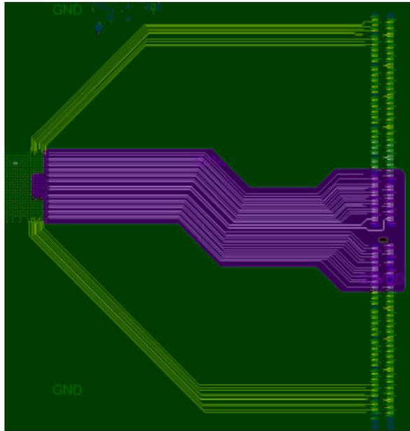
**Figure A-8. GND layer 2 with UDIMM memory**
