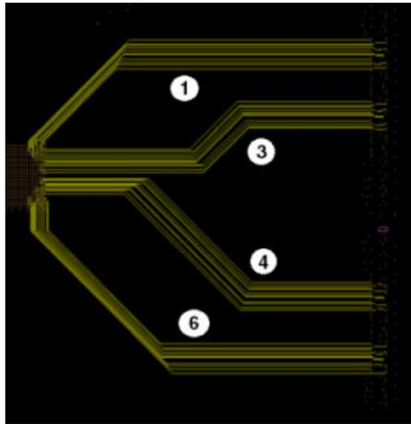
Figure A-10. Signal layer 4 with UDIMM memory
