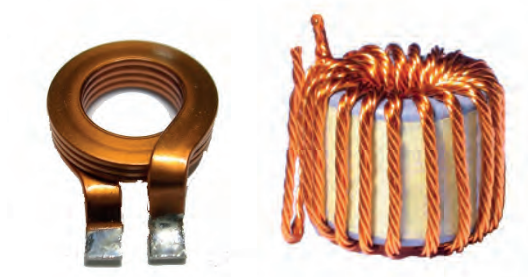
Figure 10.24: Flat wire and Litz braided wire windings
