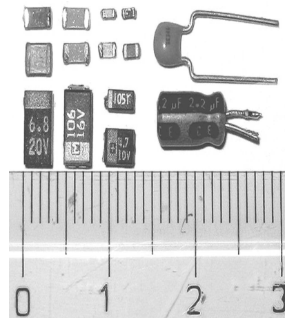
FIG. 1-12. Chip and ceramic capacitors. (Courtesy of Wikipedia)
