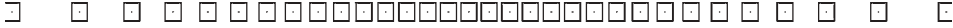
FIGURE 12-7 Locations of a 32-element space tapered line array for 30-dB Taylor distribution.
