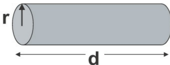
Figure 6-6 Geometry for the approximation of the partial self-inductance of a round rod. The length of the wire, d , is also represented by Len .
