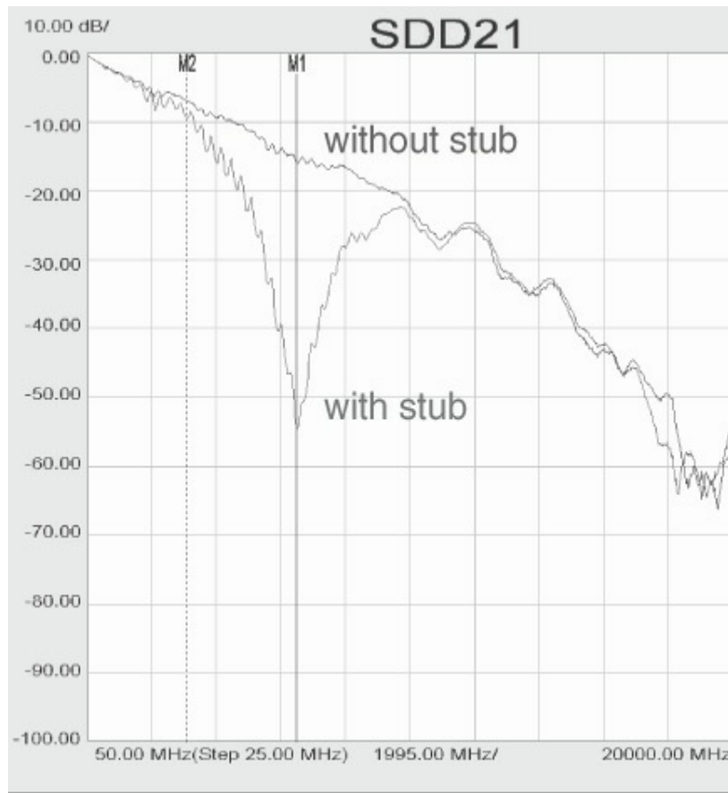
Figure 12-35 Measured differential return loss of two backplane channels, one with a 0.25-inch-long via stub and one with the via stub backdrilled. Measured with an Agilent N5230 VNA and displayed with Agilent's PLTS. Data courtesy of Molex Corporation.
