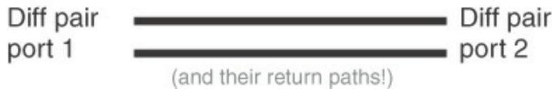
Figure 12-31 The same two transmission lines can be equivalently described as two single-ended lines with coupling or one differential pair. As one differential pair, there is one differential port on each end.
