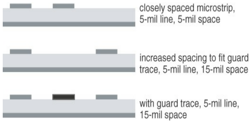
Figure 10-42 Three different microstrip structures evaluated for noise at the receiver of the victim line.
