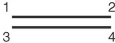
Figure 12-4 Recommended port assignment labeling scheme for multiple transmission-line interconnects. The pattern continues as additional lines are added.
