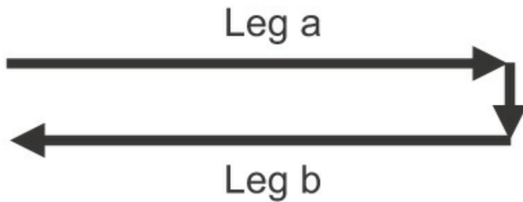
Figure 6-9 A current loop with two legs: an initial current and its return current.
