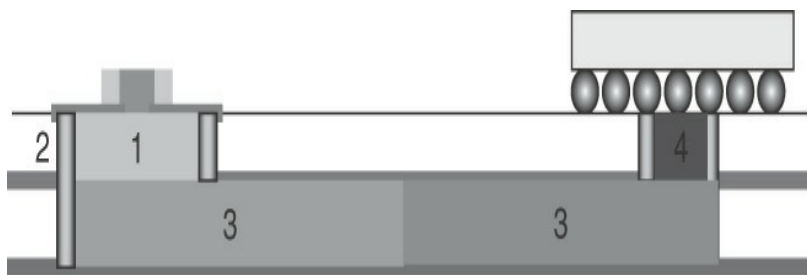
Figure 13-27 The ESL associated with a capacitor can be separated into four distinct regions.
