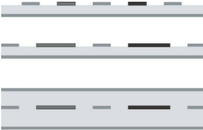
Figure 10-41 Examples of cross sections of traces that incorporate guard traces. The guard trace is hatched; all other traces are signal traces.
