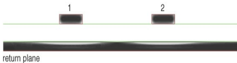
Figure 11-16 The current distribution, at 100 MHz, in a pair of coupled 50-Ohm microstrip transmission lines, 5 mils wide and separated by 15 mils. Lighter shading means higher current density. The current density scale in the plane is 10 times more sensitive than the traces to show the current distribution more clearly. Simulated with Ansoft's SI2D.
